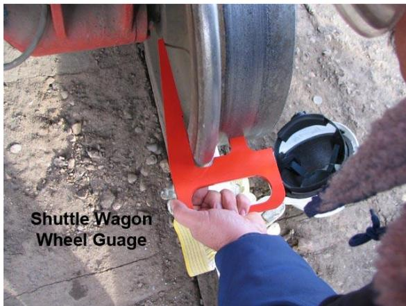
Most Shuttle Wagon wheels cannot be measured with a standard AAR wheel gauge. In order to accurately measure wheel tread wear and flange height must be made with a factory supplied wheel gauge. The use of an AAR gauge will result in inaccurate measurements and may result in premature wheel replacement. Only a competent person should use the wheel gauge.
