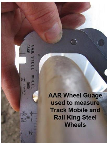
Track Mobile and Rail King rail car mover's steel wheel measurements can be made utilizing an AAR approved wheel gauge. Your rail car mover manufacture or vendor should be contacted for the appropriate gauge.
