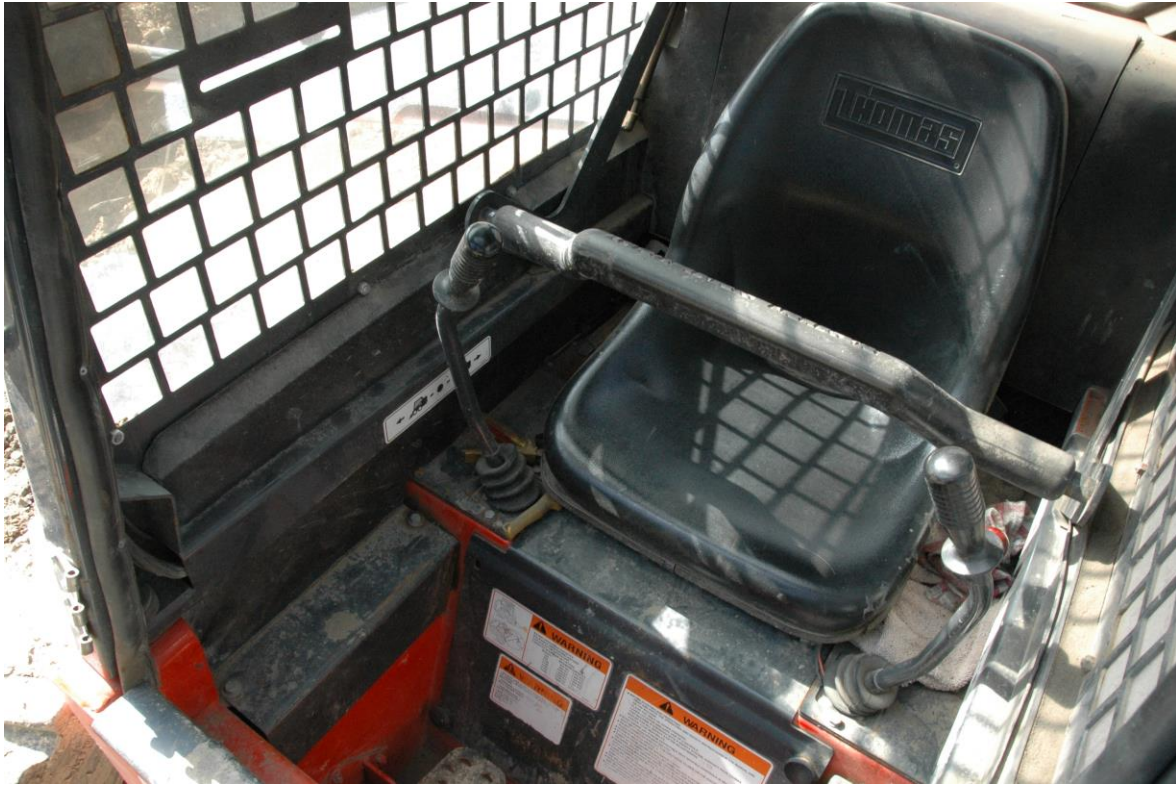
Photograph 5 – Shows the seat bar in the down position.
