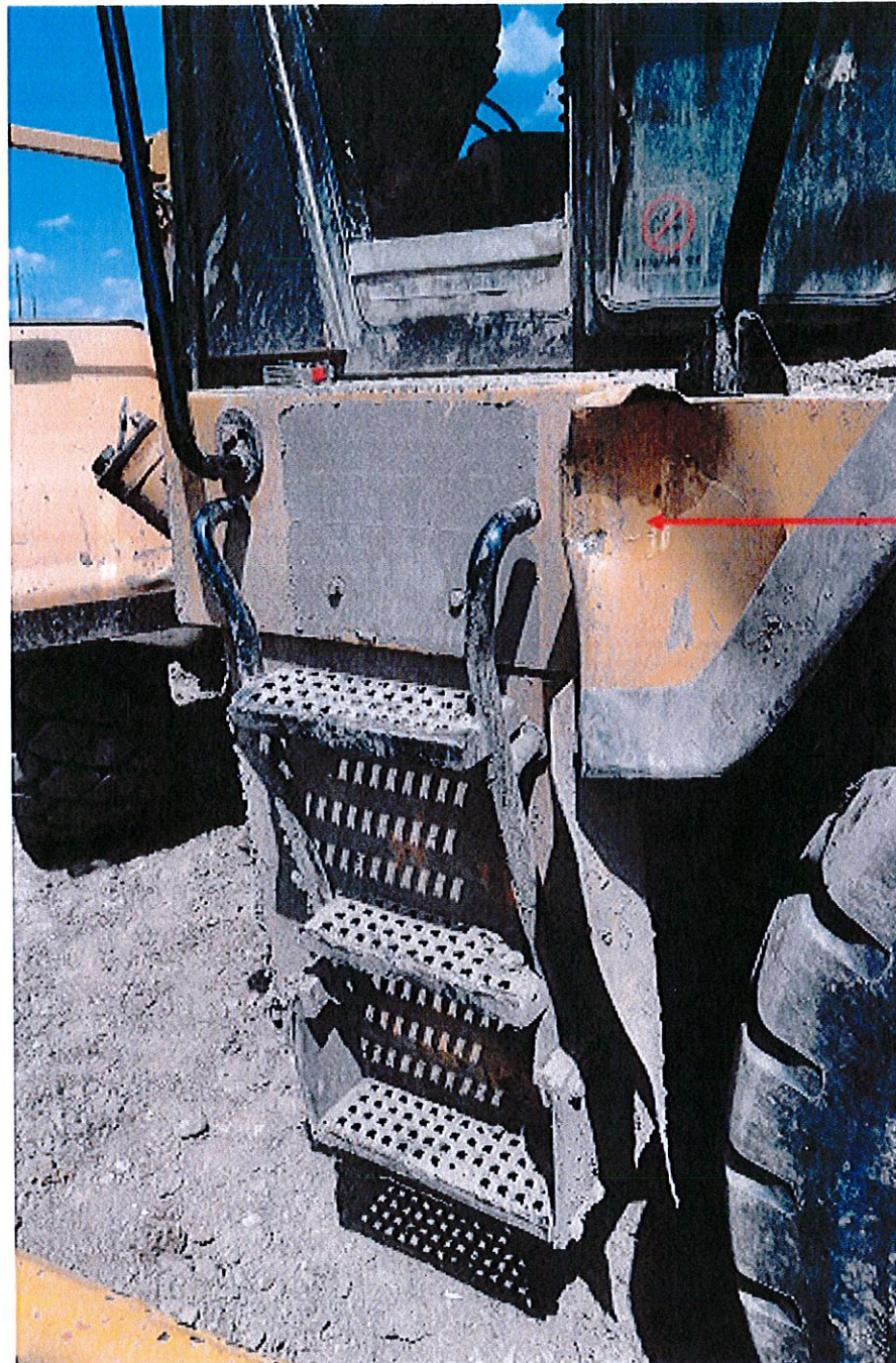
Photograph 4: Shows the side and ladder area of the wheel loader where the tracked loader backed into it
