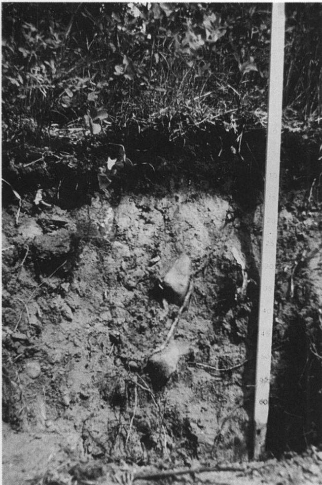
Plate 3. Soil profile of an Eluviated Black developed on till showing a 15 cm thick black coloured surface layer over a lighter coloured layer (Angus Ridge soil series).
