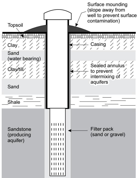
The annular seal will be disturbed during installation of the pitless adapter. It is the responsibility of the person completing this installation to re-establish the annular seal back up to ground surface.
