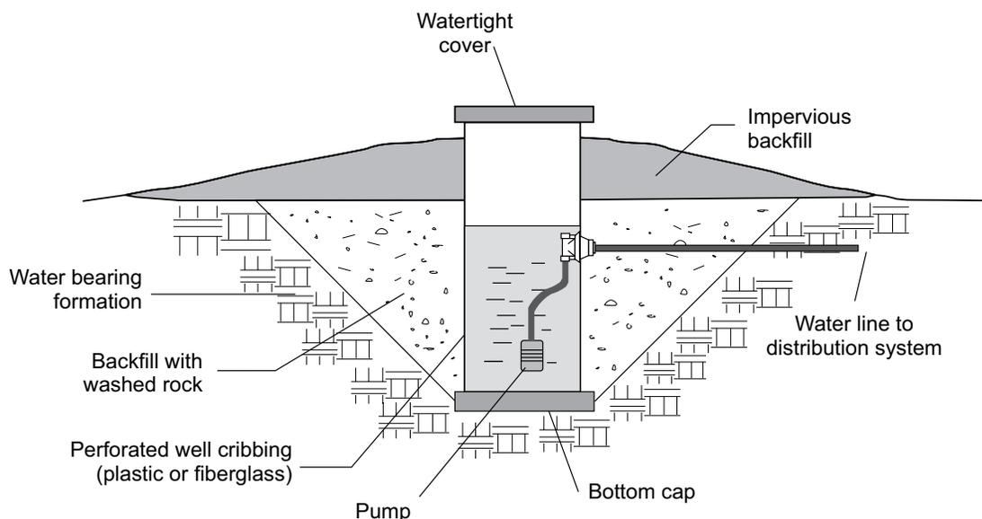
Drilled wells are smaller in diameter, usually ranging from 10-20 cm (4-8 in) and are completed at much greater depths than bored wells. The producing aquifer is typically much less susceptible to contamination from surface sources because of the depth and the water supply tends to be more reliable since it is less impacted by seasonal weather patterns. Drilled wells are constructed by various rotary or percussion drilling methods and well completions vary (see Figure 3-4, Well Completions).
