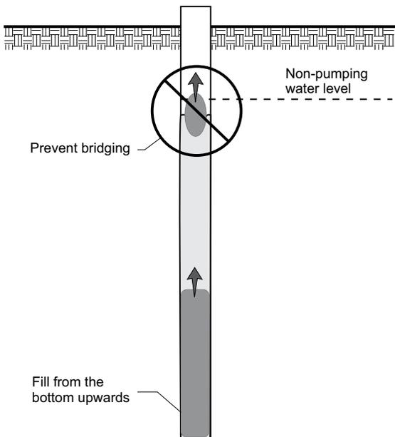
Figure 8-3, Pouring Bentonite Chips
