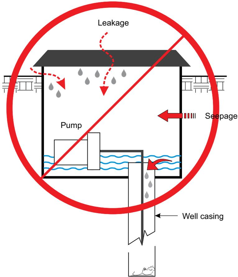
Well pits are “confined spaces” that can be a safety hazard to anyone who enters the pit. The air in the pit can become oxygen deficient or may contain dangerous gases that can come up from groundwater through the well. In Alberta, well pits have exploded due to the build-up of methane gas and people have died from asphyxiation after entering oxygen-depleted well pits.
