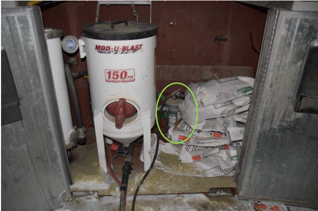
Figure 2. Mod-U-Blast Abrasive Blasting Machine and RADEX breathing air filter (indicated by green circle).
