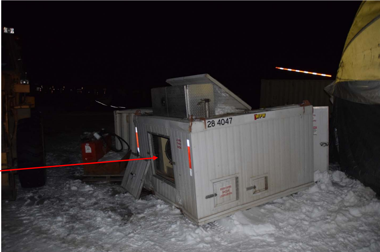
Figure 1. Abrasive blasting unit assembly (compressor, abrasive blasting unit and breathing air filter) located outside the sandblasting area. The compressor is indicated by the arrow.
