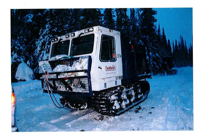
Photograph #9 Shows another shot hole drill the same as the vehicle involved in the incident.
