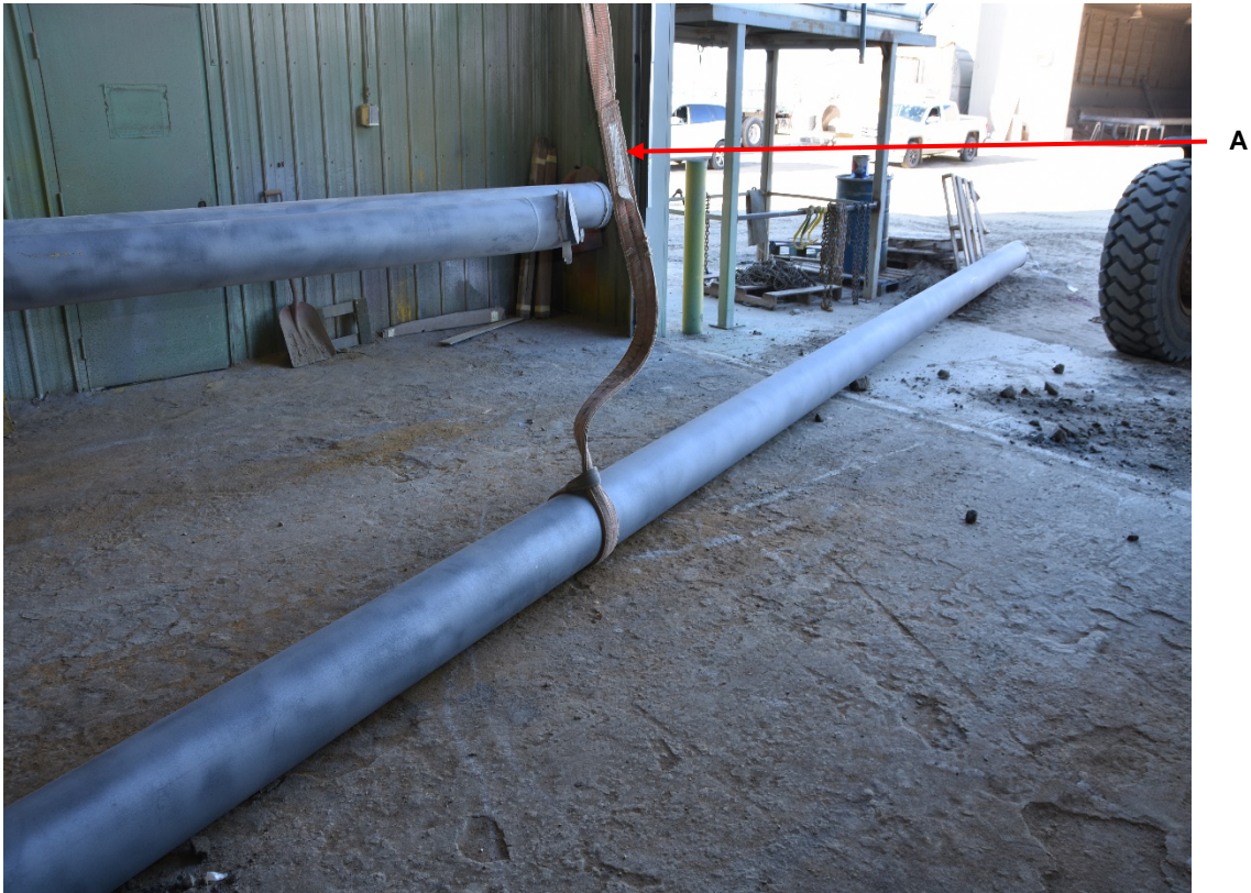
Figure 8. Synthetic fibre sling secured to pipe.
