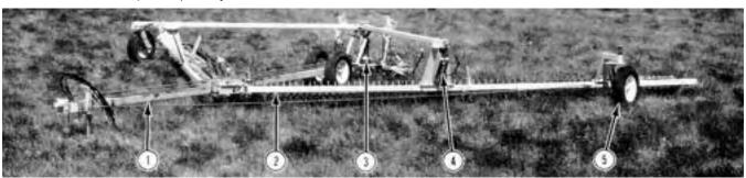
FIGURE 1. Phoenix Rotary Harrow Model HT140: 1) Hitch Frame. 2) Wing Frame, 3) Transport Motor Drive Location, 4) Tine Lift Cylinders, 5) Wing Wheels.
