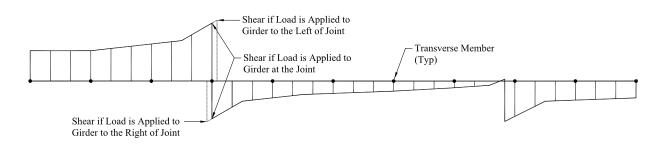
Figure F3 Shears in Loaded Girder with Continuous Transverse Members
