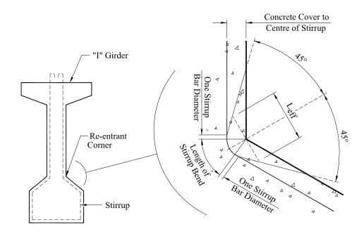
FIGURE 9.5.5.3 Determination of L<sub>EFF</sub> at Stirrup Re-entrant Corner
