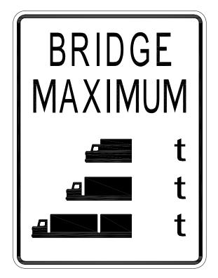
FIGURE 10 Bridge Load Posting Sign
