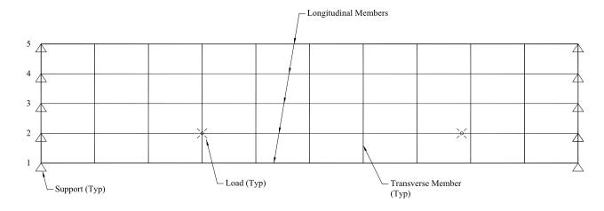
Figure F1 Grillage Analogy Model of Bridge Superstructure
