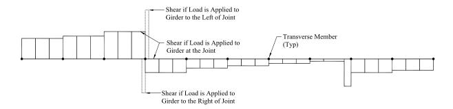
Figure F2 Shears in Loaded Girder with Discrete Transverse Members
