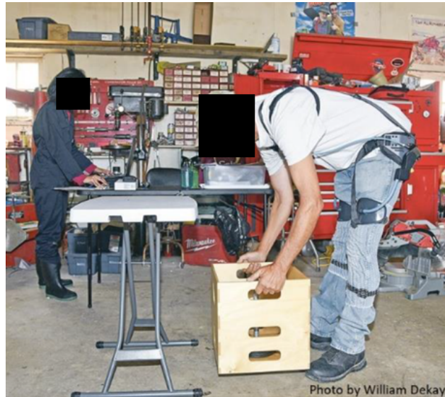
Figure 3: A farmer (R) lifts a box during the repetitive lifting standardized task while wearing the exoskeleton. Photo by William Dekay.
