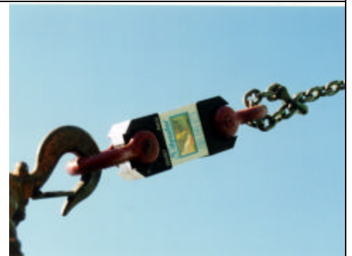
Jacking pumps require calibration and gages to monitor clamping and jacking forces that are applied. Tension forces on pullers and come-alongs can be measured with calibrated load cell devices.
