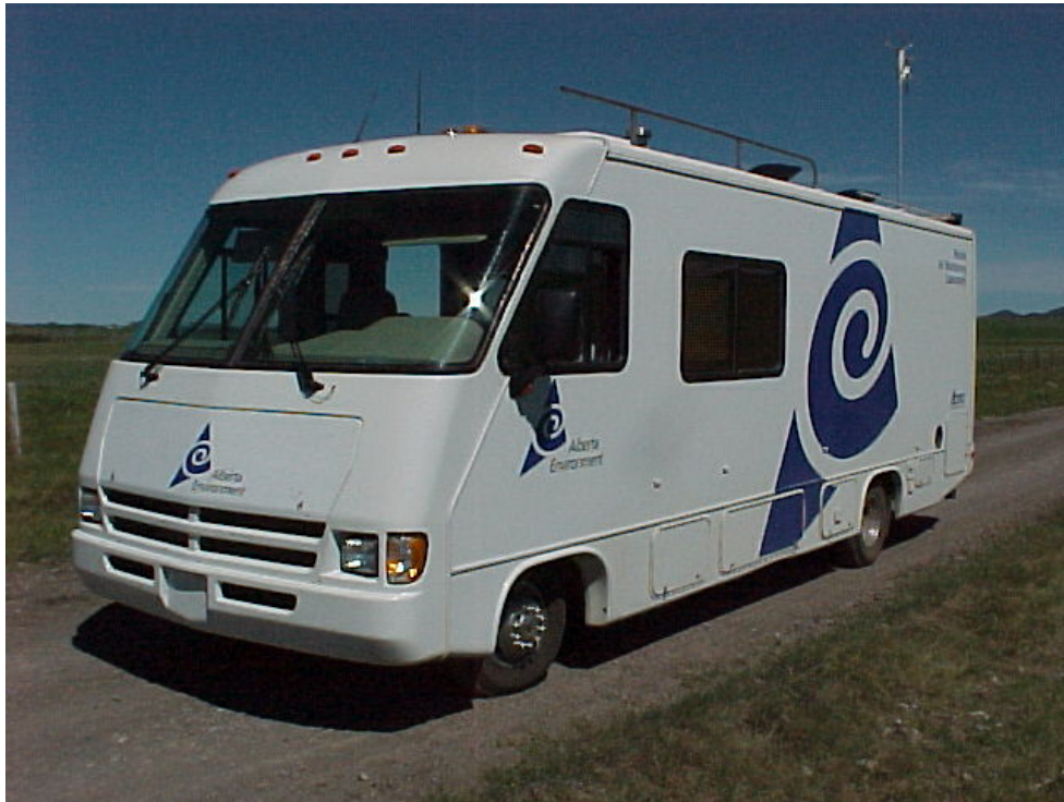
Figure B1: Alberta Environment's Mobile Air Monitoring Laboratory
