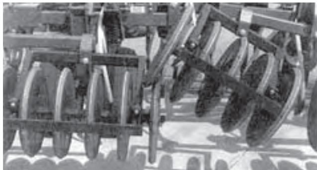
FIGURE 9. Interference between wing and main frame press wheel gangs.
