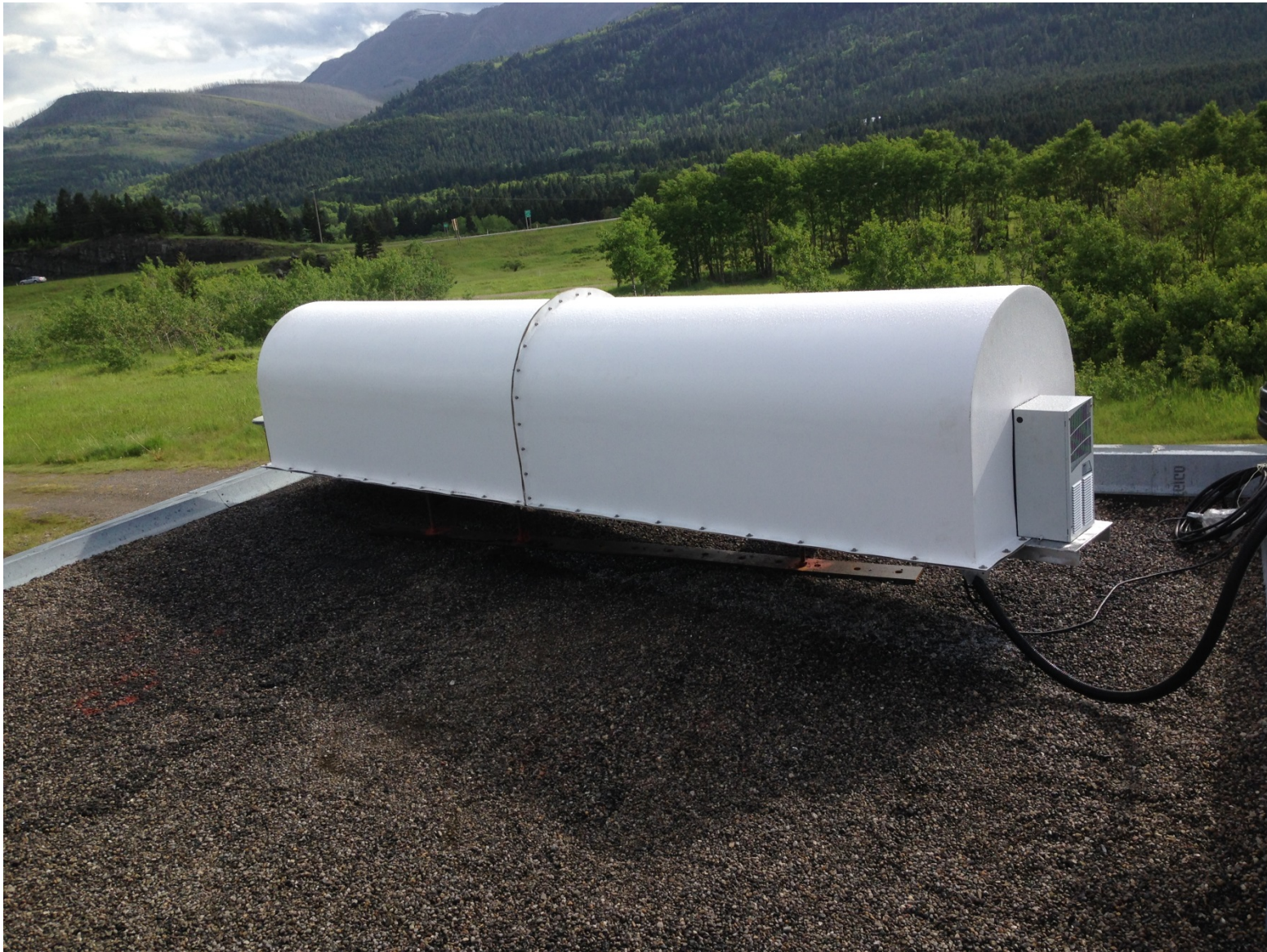
Source: AER/AGS - Ground-Based Interferometry (GBInSAR) used at Turtle Mountain
