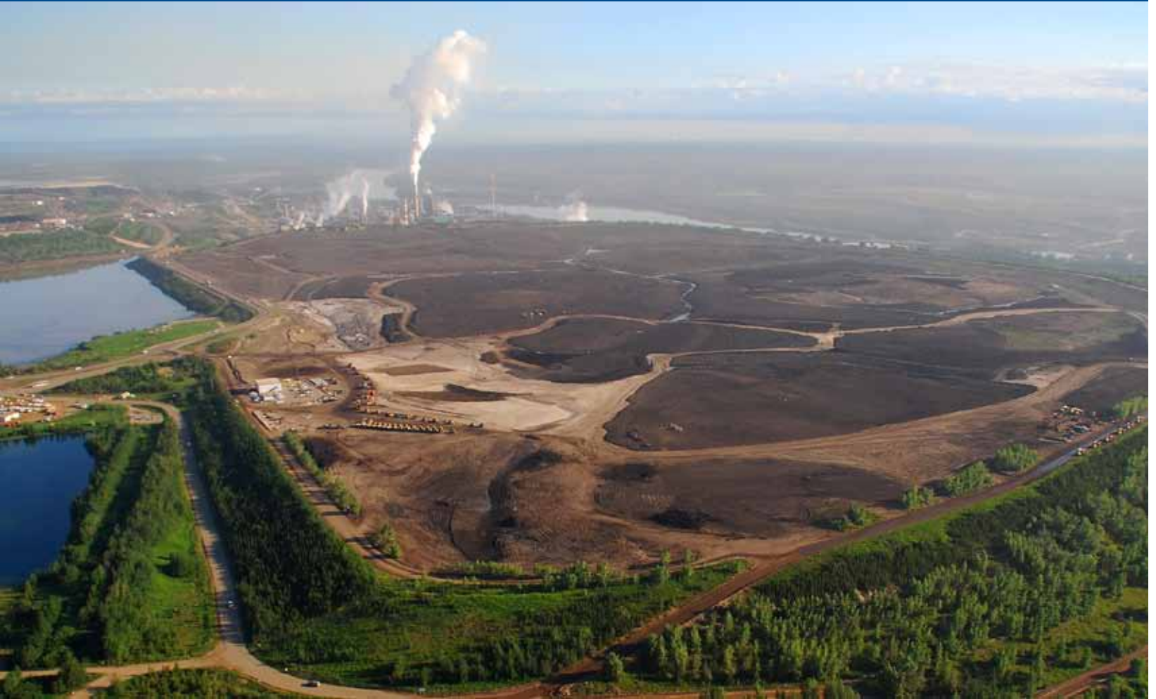
Suncor Energy's Pond I in June 2010 ▼ Suncor is the first Alberta oil sands company to convert a tailings pond to a stable surface solid enough to be re-vegetated.
