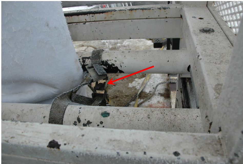
Figure 2. Ratchet strap in place on lower gland of the DGAI.
