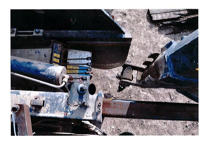
Photograph #4 Top view of knuckle boom picker controls, outrigger and boom positioned from the passenger side.
