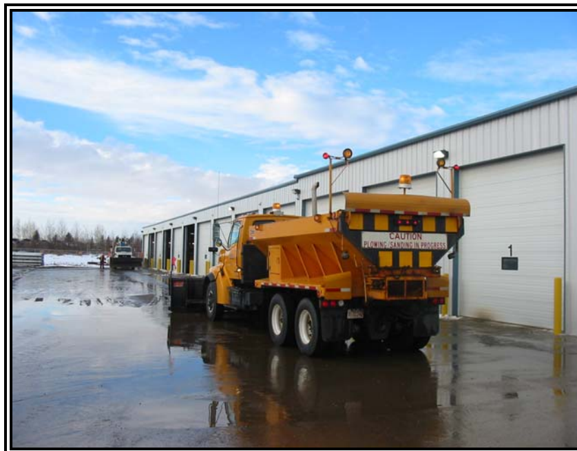
Photo #4 - Viewing the same snowplow as seen in Photo #3. From this angle the required reflective tape can be seen along the side of the snowplow as well.
