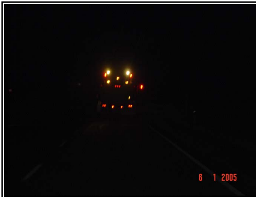
Photo #16 – Approximately 50 to 75 metres from the rear of the snowplow truck. From this distance each light can be clearly seen. The lighting configuration is slightly different from the specifications where there are two front mounted amber beacons. The elevated amber lights appear to be the brightest.
