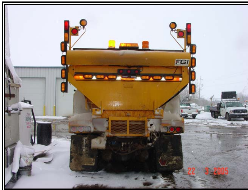
Photo #20 - This photo shows the test snowplow truck. This truck has been outfitted to accommodate all of the lighting trials (not all shown). A steel square hollow beam was used to mount a variety of beacons.
