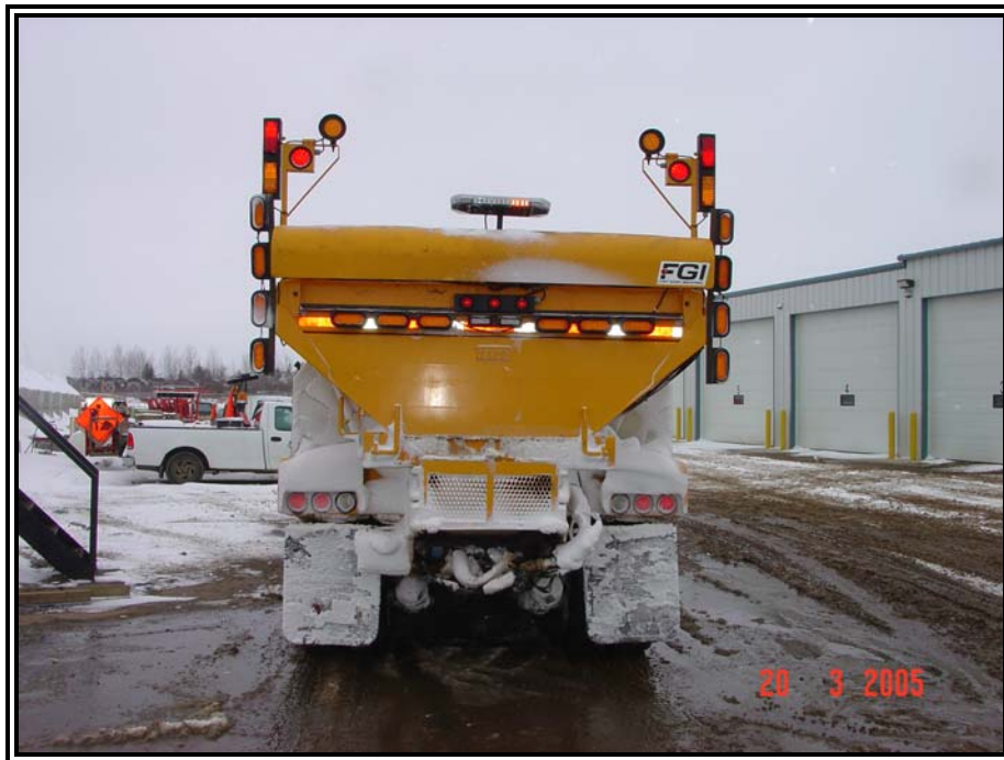
Photo #22 - This photo has been taken to show the trial snowplow outfitted with the PSE Amber 2100 low profile light bar for use as the centre beacon.
