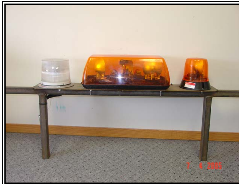
Photo #26 - This photo show the cross member used to install the warning beacons. Three (3) beacons were mounted to two (2) cross beams to allow different options to be viewed in quick succession in the field.
