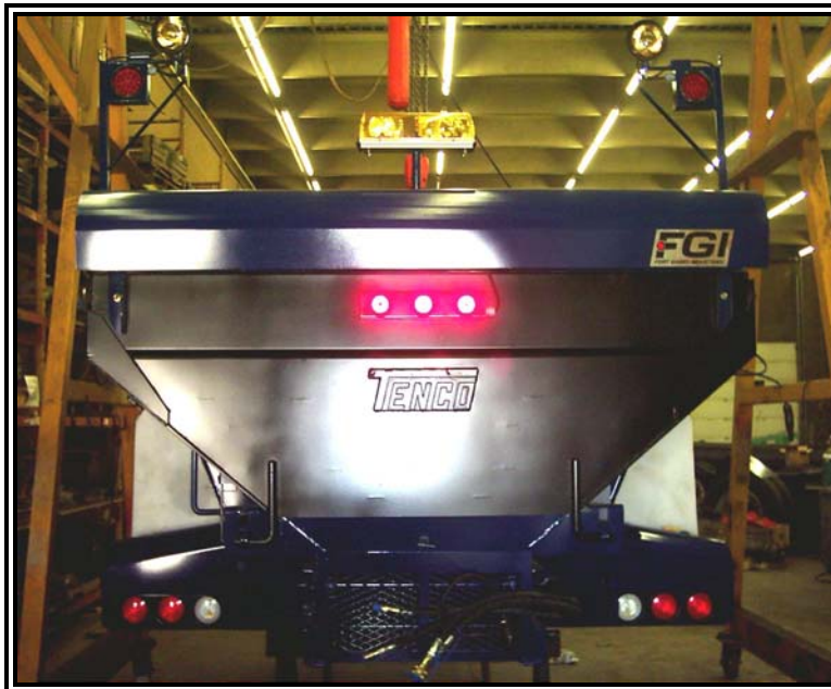
Photo #18 - This lighting setup has moved the location of the red marker lamp inside the mounting bracket and placed inside a square metal box, as seen previously in Photo #2.
