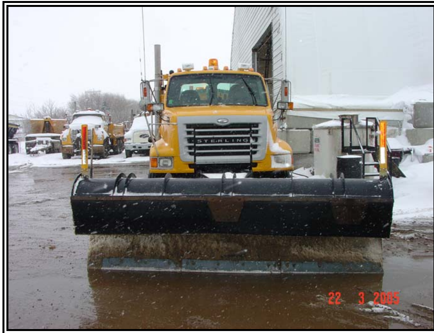
Photo #25 - Another picture from the front of the snowplow. The reflective striping on both corners of the plow can be seen here. A rubber skirt has also been added to the plow blade to help reduce the snow that comes over the truck. A single amber beacon is used on the front of the truck, mounted on the cab.
