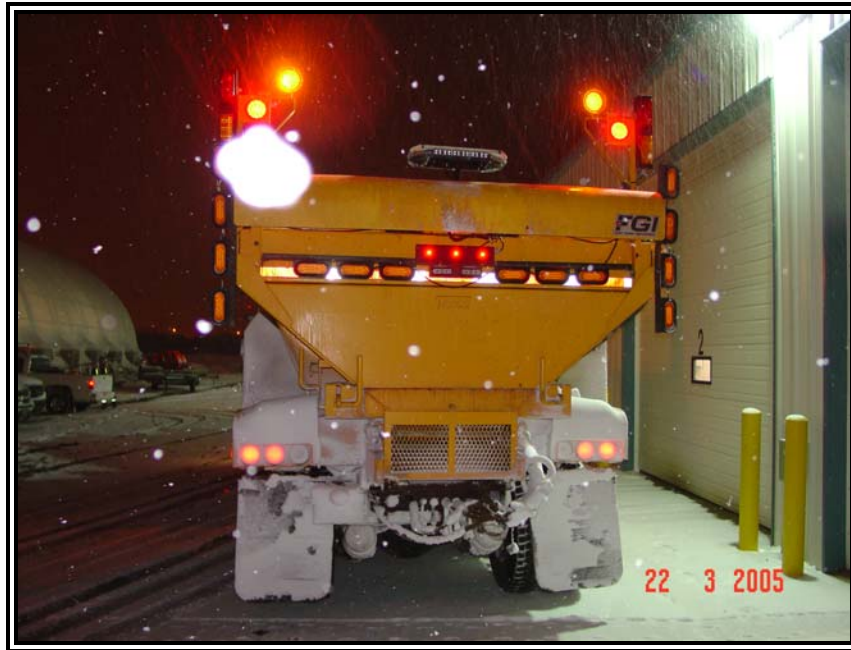
Photo #35 - The existing tail, brake, rear ID and elevated warning lights were replaced with LED lights for the field trials. These lights can be seen in the above photo.
