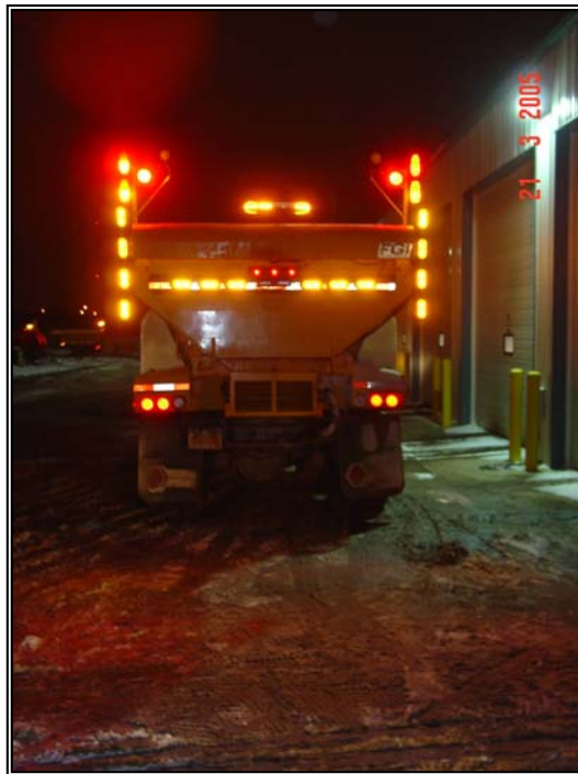
Photo #36 - This photo shows the entire trial configuration turned on at once. Amber-red LED flashing warning lights, vertical and horizontal lights bars and directional LED were all tested.
