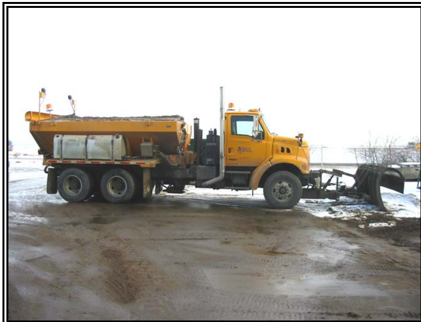
Photo #6 - A side view of a snowplow. In this photo the wind deflector, used to keep the rear of the truck clear of snow buildup, can be seen. Also, de-icing tanks are being used and are located on the sides of the truck. A front flashing amber beacon and additional headlights are also used.
