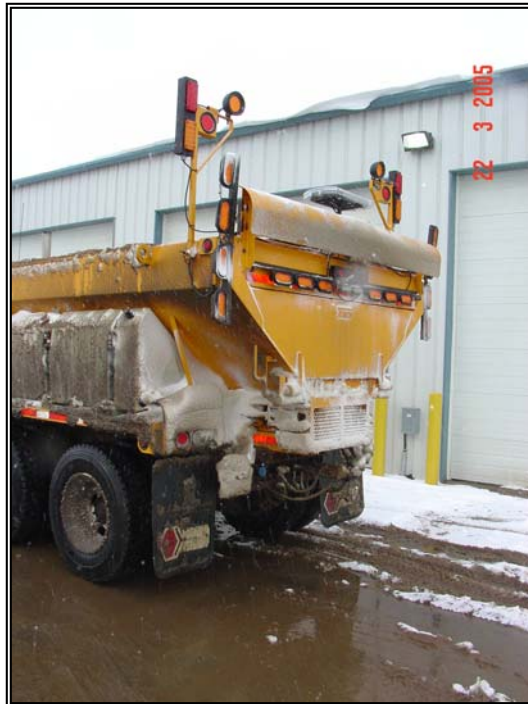
Photo #30 - This photo taken at the same stage of the trials as above shows that snow has not only accumulated on the wind deflector but on the vertical LED light bars as well.
