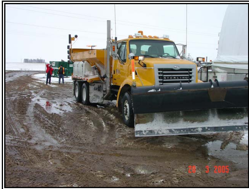
Photo #24 - Viewing from the front corner of the trial snowplow. The vertical reflective strips, which have been mounted on each corner of the snowplow blade, can be seen in this photo.
