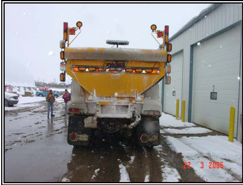
Photo #29 - This photo of the trial snowplow truck, outfitted with the low profile light bar as the centre beacon. Snow has built up on the upper wind deflector; however, the wind deflector has kept the back of the plow clear.
