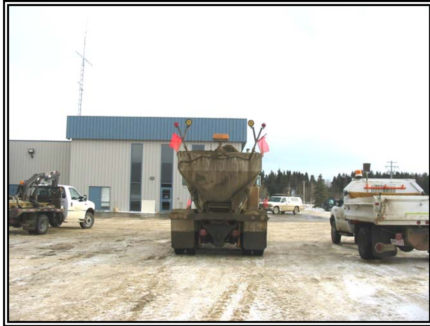
Photo #9 - Viewing an alternate lighting setup used by Parkland County. In this configuration orange warning flags have been installed to compliment the elevated amber and red warning lights. A dual amber rotating beacon is being used above the box.
