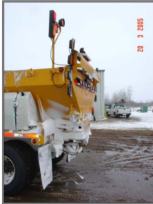
Photo #23 - A side view of the field trial snowplow truck. Snow buildup can be seen on the wind deflector over the Stop-Tail-Turn and backup lights and the side of the truck box. The wind deflectors are not properly working over the tail lights as de-icing tanks are mounted along the box.
