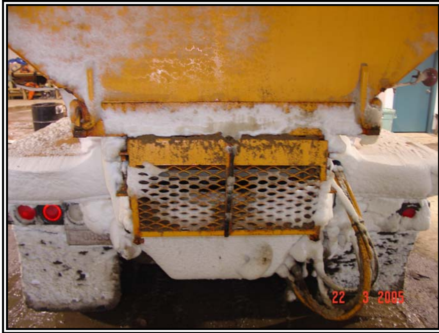
Photo #33 - This photo shows a direct comparison of the effectiveness of the wind deflectors on each side of the snowplow. In summary, the lower wind deflectors appear to be not working.
