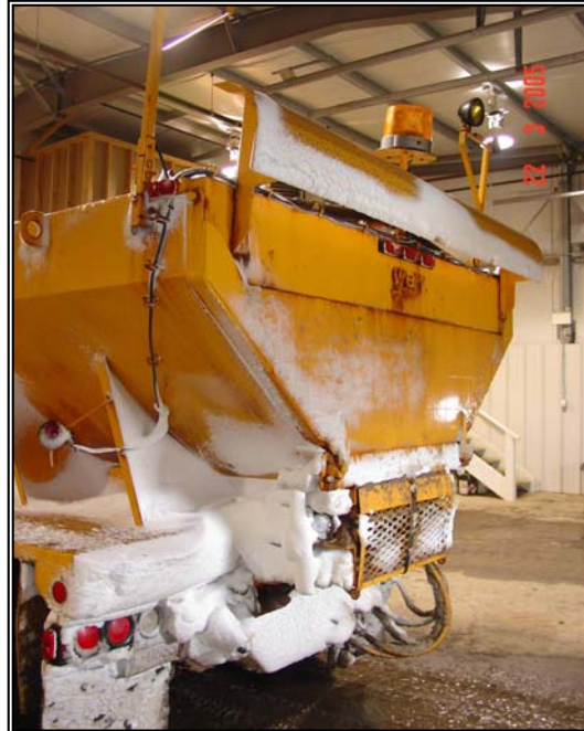
Photo #31 - This photo show extensive snow accumulation on the rear of a typical snowplow truck, when no de-icing tank is used.
