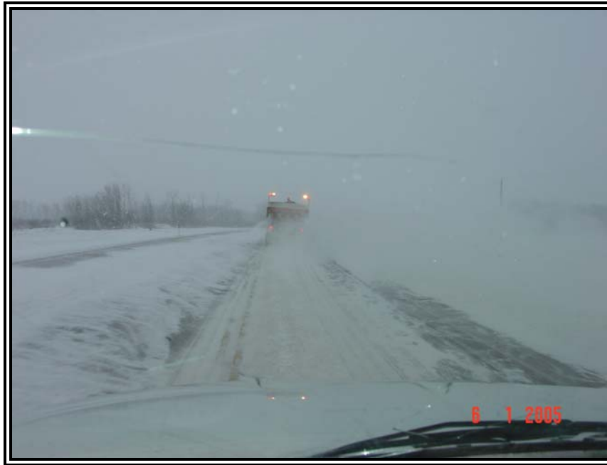
Photo #11 - A photo of a snowplow truck during plowing operations on January 6, 2005, east of Vegreville on Hwy. 16. In this photo the elevated flashing amber lights are the most visible of the rear warning lights.
