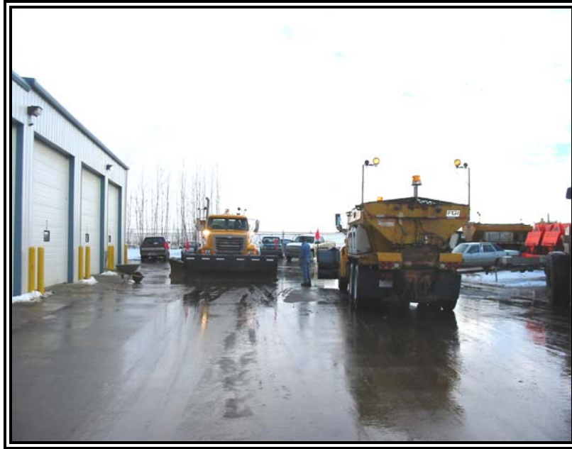
Photo #1 - A view of the existing front and rear standard lighting of typical snowplow trucks. Note that the truck on the right does not comply exactly with the Alberta Infrastructure and Transportation Highway Maintenance Specification, as the top 2.5" red warning light should be mounted sideways on the outer edge.
