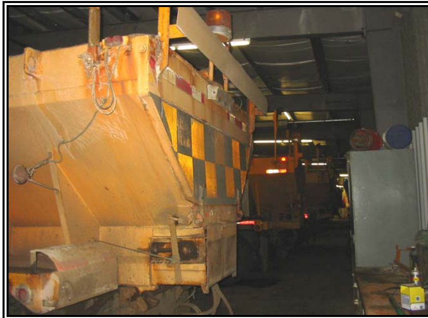
Photo #8 - This close-up of the rear of the snowplow truck shows the setup of the wind deflectors above the box and over the tail lights. The Rear Identification Lamps can also be seen below the wind deflector.
