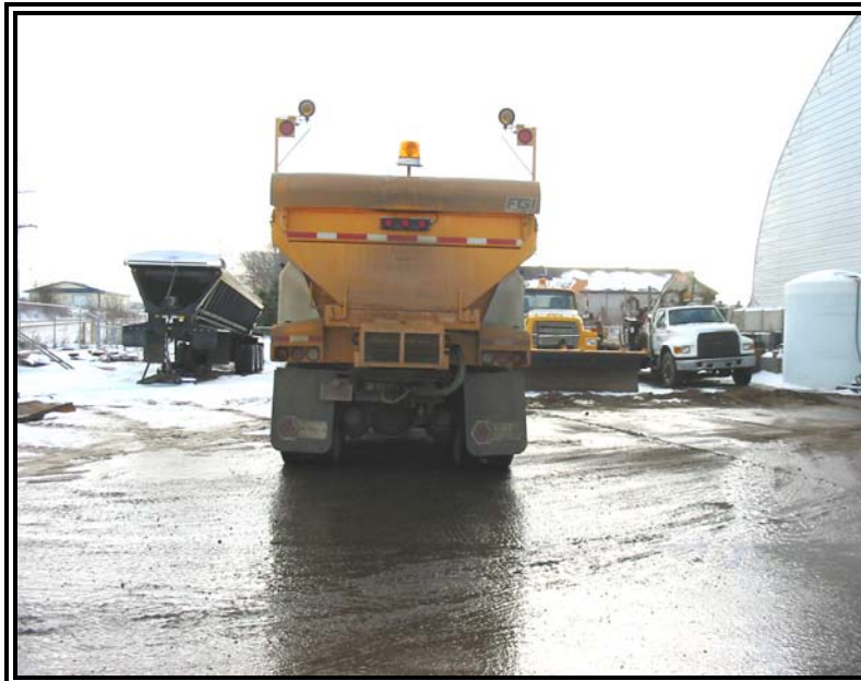
Photo #2 - Another photo of the rear lighting on a snowplow truck. Again, the red warning lights are mounted on the inside of the mounting bracket inside of on the outside as per specification. The height of the amber and red warning lights also appear to be lower for this truck.
