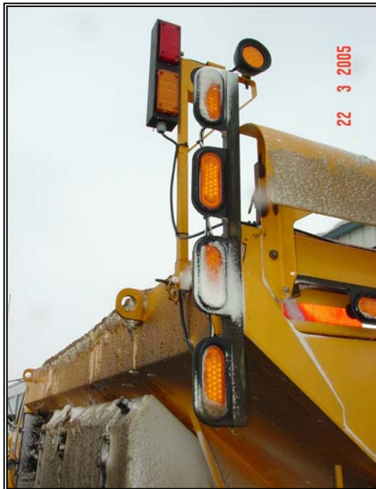
Photo #33 - This photo shows a direct comparison of the effectiveness of the wind deflectors on each side of the snowplow. In summary, the lower wind deflectors appear to be not working.
