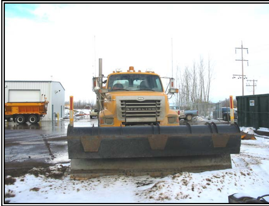
Photo #7 - Viewing the front of a snowplow. The rotating beacon required on the front of the plow can be seen in this photo. This plow has been outfitted with metal strips with reflective tape for marking the corner of the plow, in lieu of orange flags. Additional elevated headlights are also included to aid the driver.
