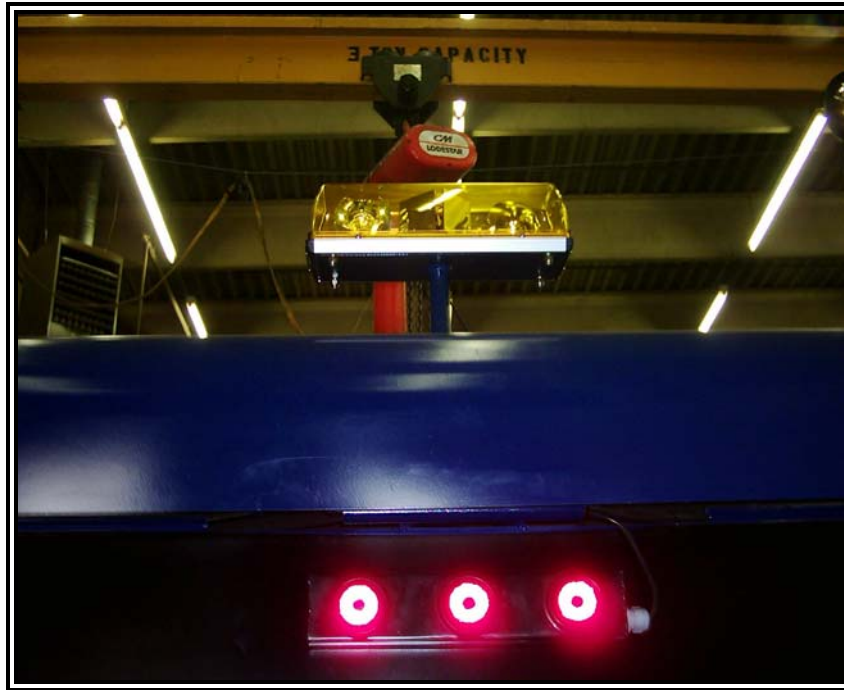
Photo #19 - The warning beacon is a dual amber Whelen beacon. This appears to be a Responder Series, R2HD, with 92,000 beam candle power from 50 Watt bulbs.
