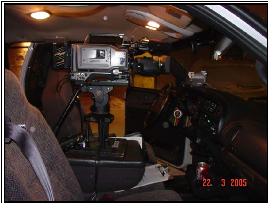
Photo #28 - The video camera was mounted to the centre console of the lead chase vehicle, a 1999 Dodge Ram 4x4. This setup allowed the camera an unobstructed view out the windshield. A second home video camera was set on the dash, as backup video coverage.
