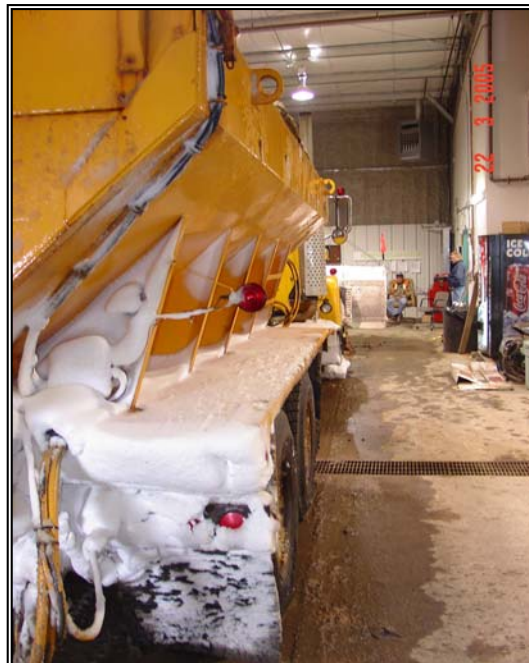
Photo #31 - This photo show extensive snow accumulation on the rear of a typical snowplow truck, when no de-icing tank is used.
