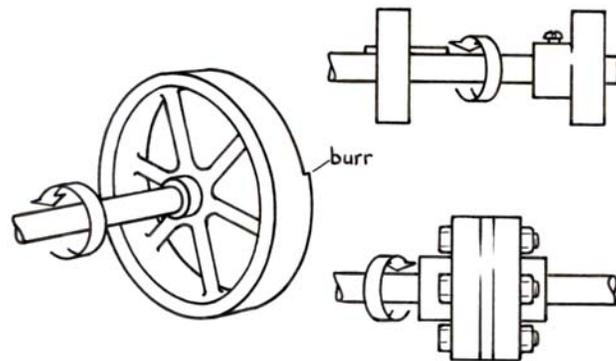
Figure 22.2 Common nip points on rotating machinery
