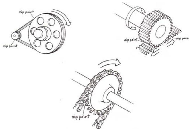
Figure 22.4 Nip points between rotating machine components
