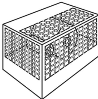
(2) Moveable guard with interlock switch
