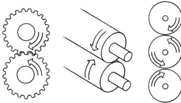
Figure 22.3 Nip points between rotating parts and parts with linear motion
