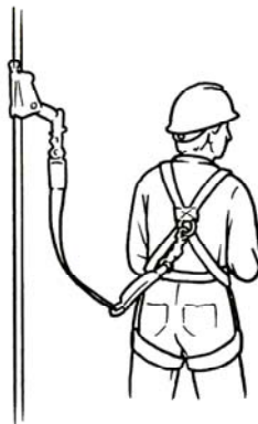
Figure 9.8 Example of a fall arrester in use
