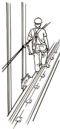
Figure 9.15 Example of using a flexible horizontal lifeline to safely move through a work area
