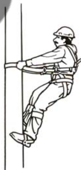
Figure 9.13 An example of fall restrict equipment used when working on or from a wood pole
