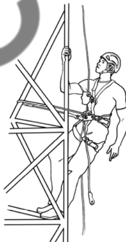
Figure 9.22 Worker on communication tower using tower climbing harness and work positioning system
