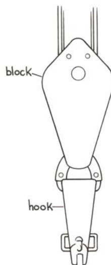
Figure 37.9 Example of a travelling block and hook
