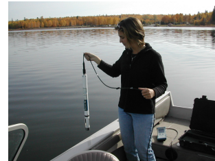
Measuring select water quality variables at a profile site using an electronic meter
