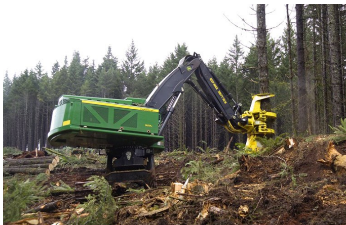
Figure 3. A feller buncher used for timber harvesting
