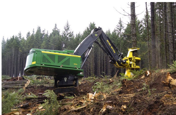
Figure 3. A feller buncher used for timber harvesting
