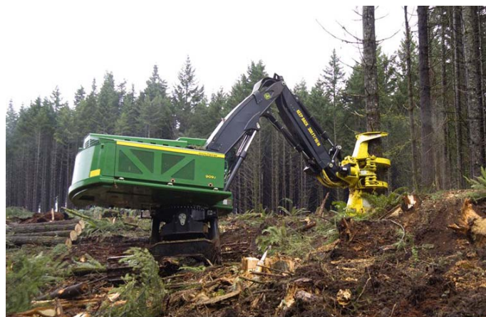
Figure 3. A feller buncher used for timber harvesting
