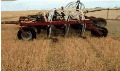
Direct seeding drills can seed into standing stubble.
