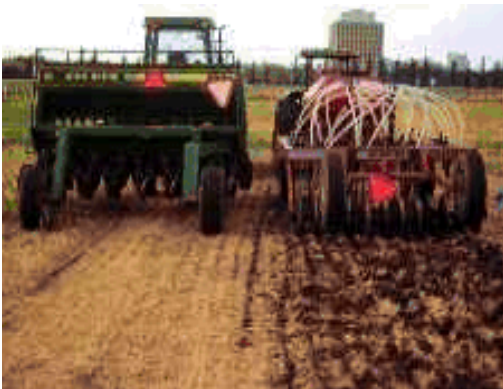
Both a disc drill (left) and an air drill (right) work well for direct seeding into sod.
