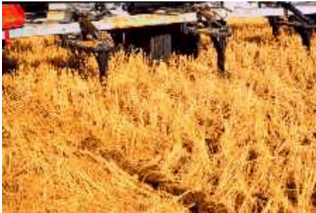
A wide blade cultivator maintains a good crop residue cover.
