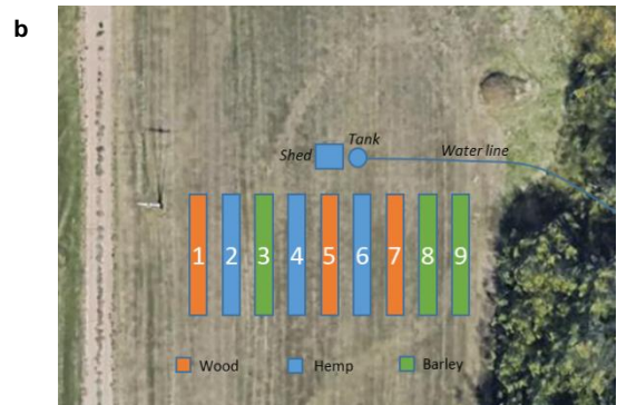
Figure 1. (a) Bioreactors at CDCN (b) CDCN Bioreactor identification and feedstocks schematic.
