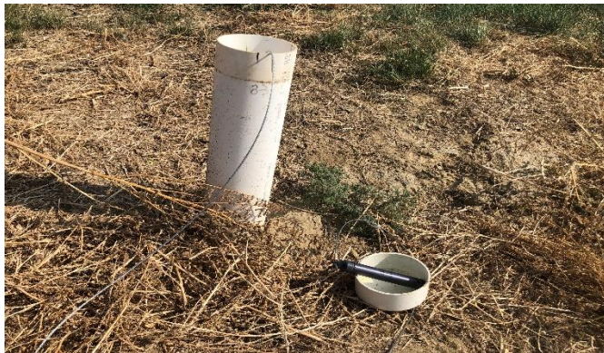
Figure 3. Sampling well with pressure transducer removed and resting on cap awaiting download.
