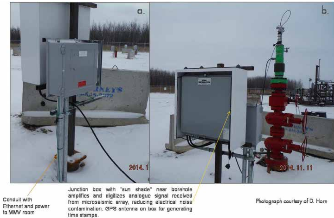
Figure 2-3: a) Ethernet connection to the on-site MMV room. b). Analogue cable exiting the wellhead and the junction box that digitizes the analogue microseismic data.
