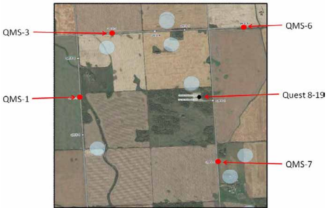
Figure 4-1: Vibroseis shot locations for sensor orientation around well DMW 8-19.
