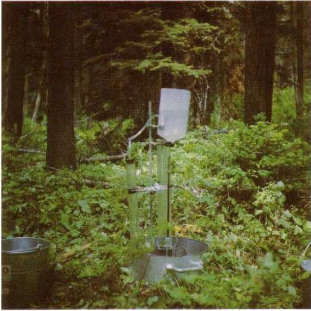
Figure 29. Field testing of water infiltration rates.
