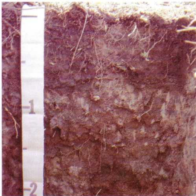
Figure 43. Soil profile of map unit 42, showing low amount of coarse fragments and high rooting volume.
