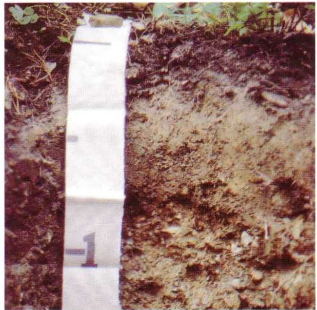
Figure 44. Soil profile of map unit 46; note pale color of the Ae horizon.
