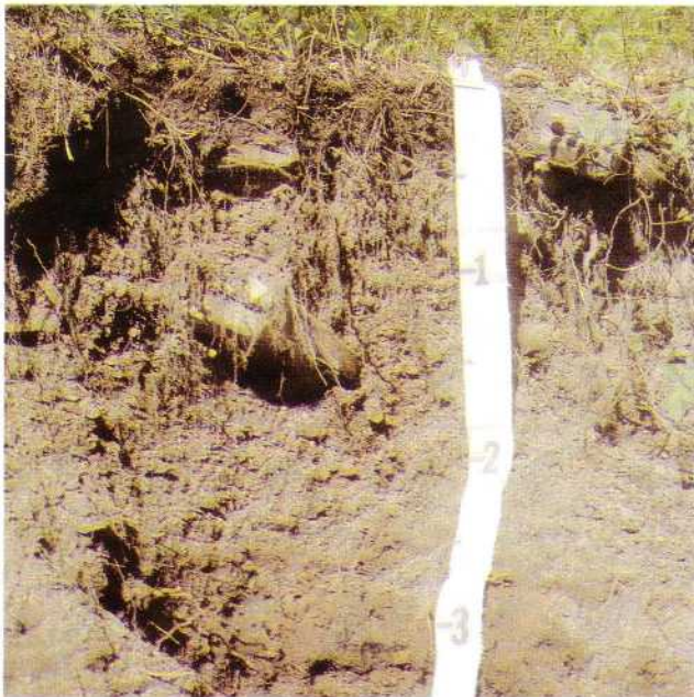
Figure 39. Soil profile of map unit 27, with silty layer at 3 feet from the surface.
