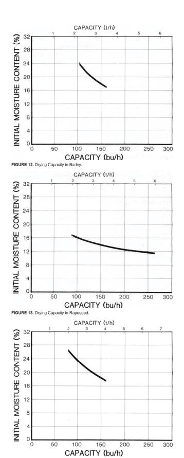
FIGURE 14. Drying Capacity in Com (Hybrid 3996).
