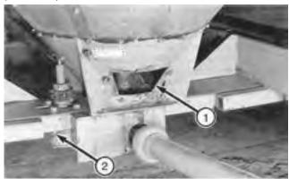
FIGURE 9. Servicing: (1) Cleanout Door, (2) Limited Access for Servicing Gear Boxes.
