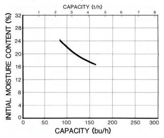
FIGURE 11. Drying Capacity in Wheat.
