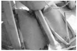
FIGURE 10. Fines Accumulated Under the Dryer.
