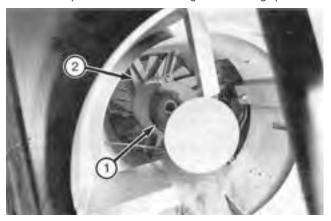
FIGURE 3. Fan Housing: (1) Burner, (2) Fan.
