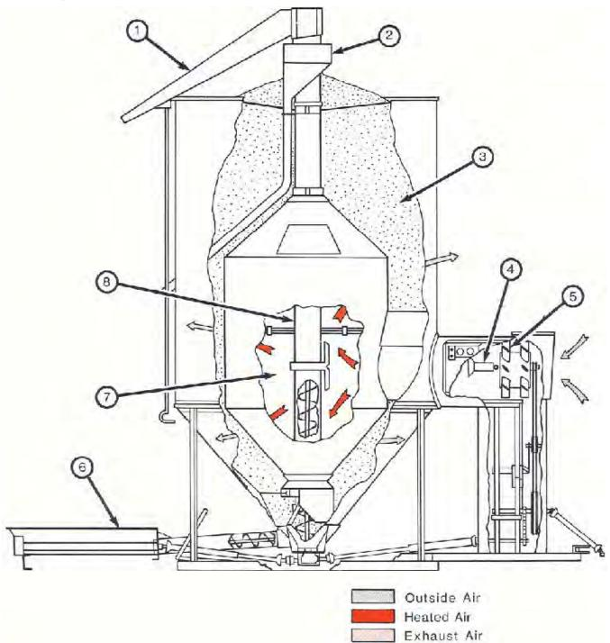
FIGURE 1. Moridge 8440 Grain Dryer: (1) Unloading Chute, (2) Grain Cleaner, (3) Grain Chamber, (4) Burner, (5) Fan, (6) Loading Auger, (7) Air Plenum, (8) Vertical Auger.
