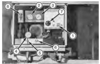
FIGURE 5. Controls and Instruments: (1) Power Switch, (2) Drying Air Temperature Gauge, (3) Grain Temperature Gauge, (4) Fuel Pressure Gauge, (5) Pressure Regulator Valve, (6) Grain Dryers. Modulating Valve, (7) Timer, (8) High Limit Switch.
