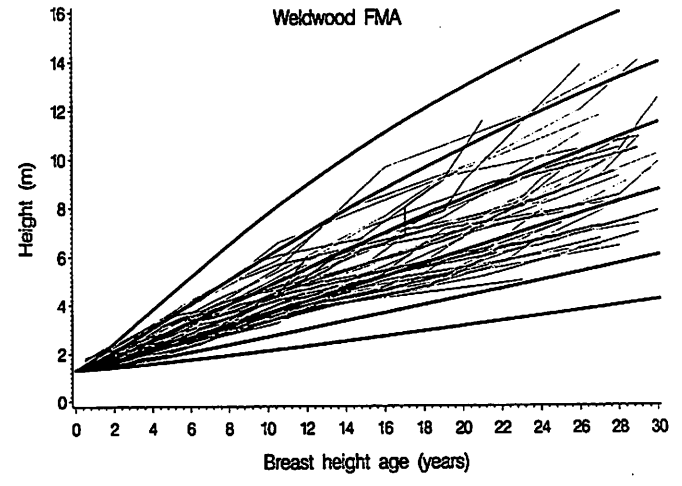
Figure 10. The growth intercept-based site index curves overlaid on observed height growth trajectories. The growth intercept-based site curves were generated using equation [1] with a base height of 1.3 m and a t value of 3-years.
