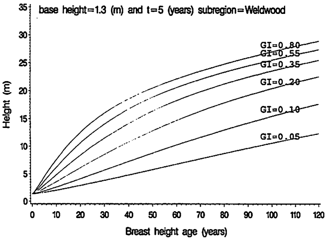
Figure A6. The growth intercept-based site index curves for the Weldwood FMA, generated from equation [1b]. Estimated coefficients are shown in Table A1.
