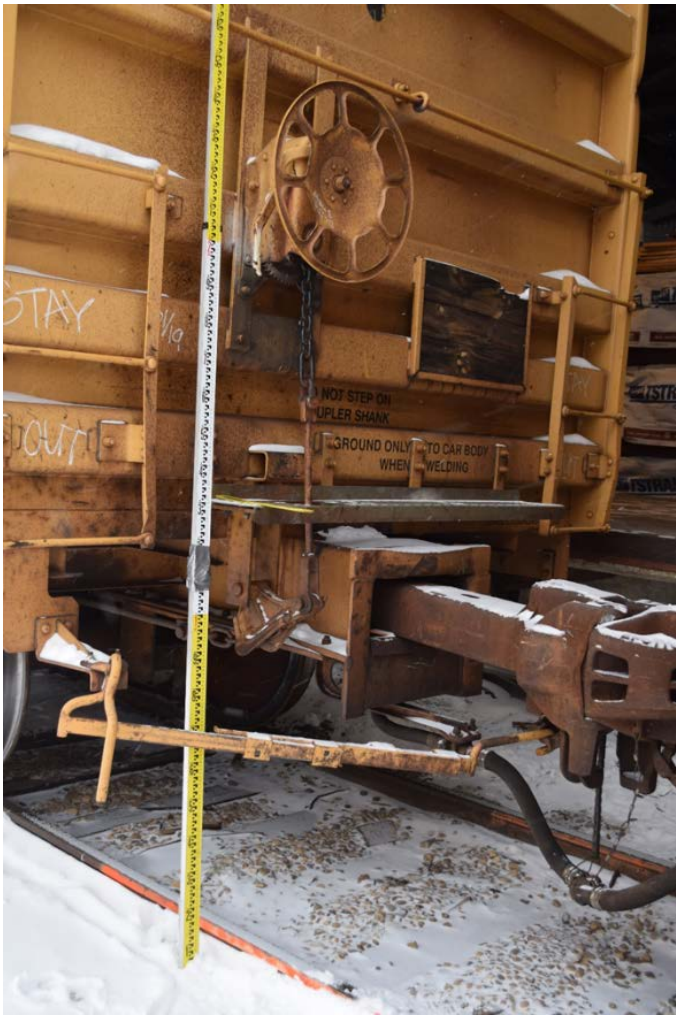
Figure 6. Work area of rail car 2 with scale. Each section of the survey measurement stick indicates 1 metre. The platform measured 1.3 metres from the ground.
