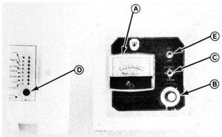
FIGURE 3. Control Box: (A) Loss Meter (B) Calibration Control (C) Sensor Selector Switch (D) Sensitivity Control (E) Power Switch.
