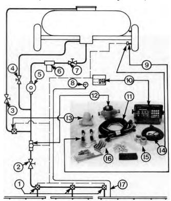
FIGURE 1, Raven Automatic Spraver Control System: (1) Solenoid Valves, (2) Throttling Valve, (3) By-Pass Valve, (4) Agitator Valve, (5) Pump, (6) Filter, (7) Shut-Off Valve, (8) Pressure Gauge, (9) Speed Sensor Magnets (10) Control Console, (11) Cables with Pull-apart and Screw-on Polarity Connectors, (12) Flow Meter, (13) Motorized Control Valve, (14) Speed Sensor Switch Assembly, (15) Flow Meter Pipe Couplers, (16) Mounting Hardware, (17) Boom Pressure Line.
