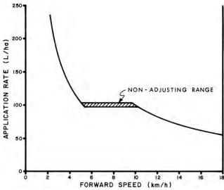
FIGURE 6. Application Rate at Various Forward Speeds with the Automatic Sprayer Control System in the Automatic Mode with an Increased Preset Pressure Range.
