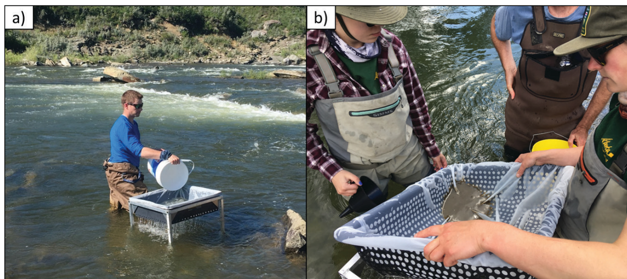
Figure 3: Field water filtrations were used to assess TAM density in the Crowsnest River. Crews poured approximately 1900 L of stream water through a 20 µm polyester screen (a) and rinsed the filtrate into a 500 mL container (b).
