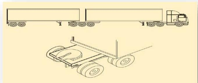
*B train - example of a unit connected by a type B converter dolly.*
