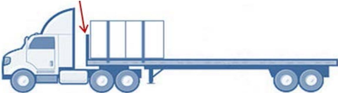
It is important to note that a cab shield is not a front-end structure or part of the cargo system
