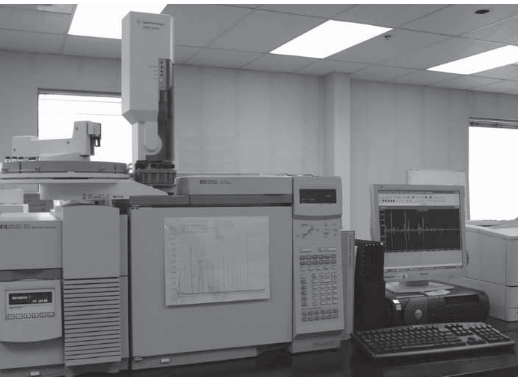
Gas chromatography-mass spectrometry equipment used to identify accelerants used in arson.
