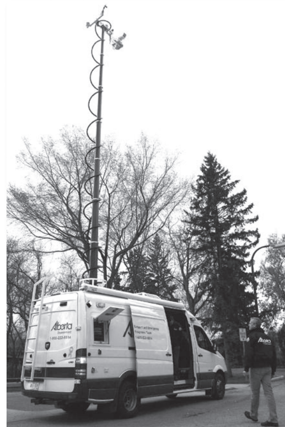
Sprinter mobile operations unit with boom fully deployed facilitating aerial incident overview and meteorological conditions.
