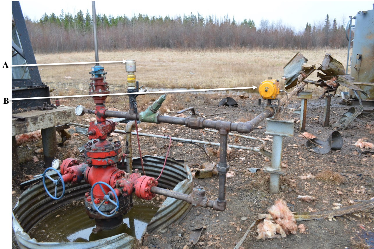
Figure 2. The pressure switch and ESD. Post incident showed that the pressure switch and the ESD were both engaged prior to incident occurring.
