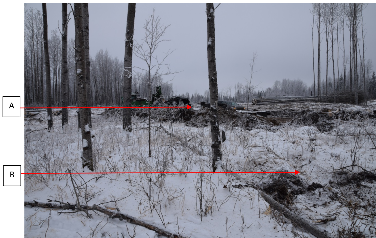
Figure 4. View from feller/buncher to truck-trailer. Indentation is consistent with a fallen tree from the feller/buncher.
