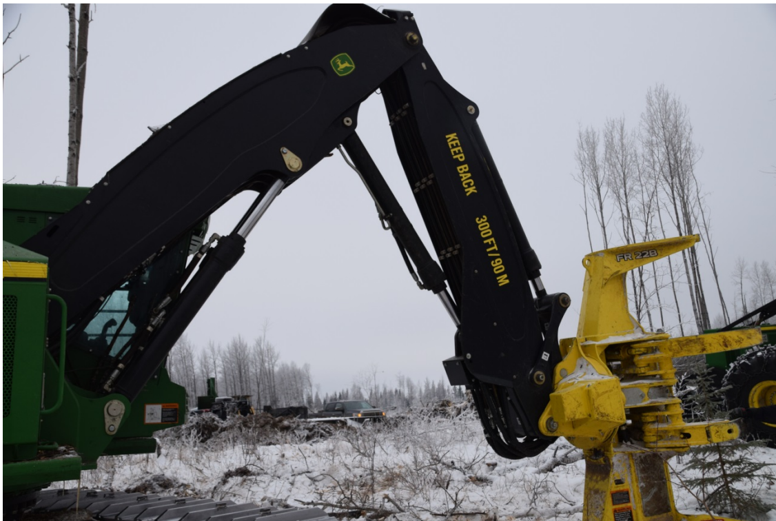
Figure 3. Feller/buncher. Proximity warning can be seen on the boom.
