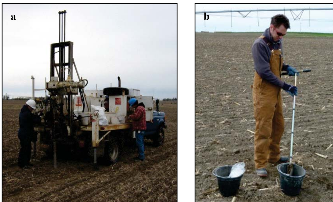
Figure 2.27. Soil sampling with (a) a truck-mounted, hydraulic coring unit and (b) a Dutch auger.
