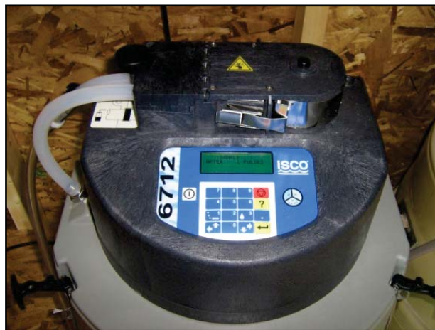
Figure 2.22. Model 6712 Isco water sampler for automated collection of water samples.
