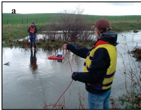
Figure 2.21. Flow metering using (a) a StreamPro with rope system and (b) wading instream with a FlowTracker.
