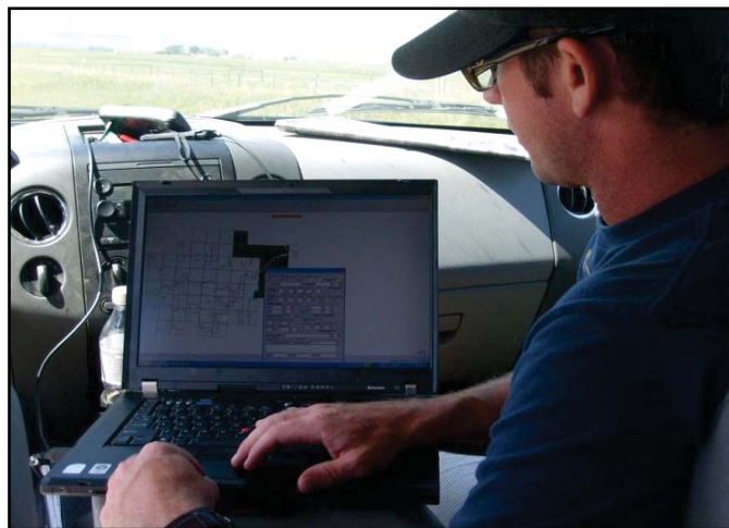
Figure 2.5. Collecting land-cover information during a windshield survey using AgCapture, a laptop computer, and GPS unit.
