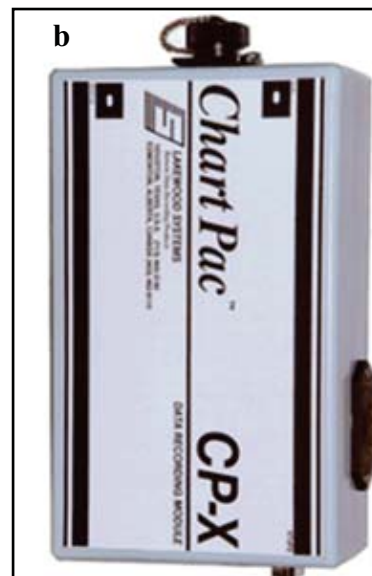
Figure 2.15. Water stage in the circular flumes was recorded using (a) two float potentiometers, with one connected to a (b) Lakewood datalogger used as a backup
