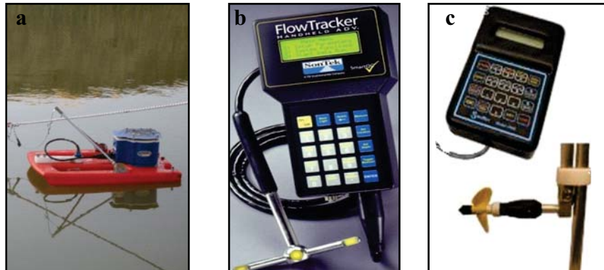
Figure 2.20. Equipment used for flow metering: (a) StreamPro, (b) FlowTracker, and (c) Swoffer velocity meters.
