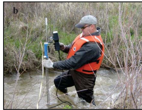
Figure 2.21. Flow metering using (a) a StreamPro with rope system and (b) wading instream with a FlowTracker.
