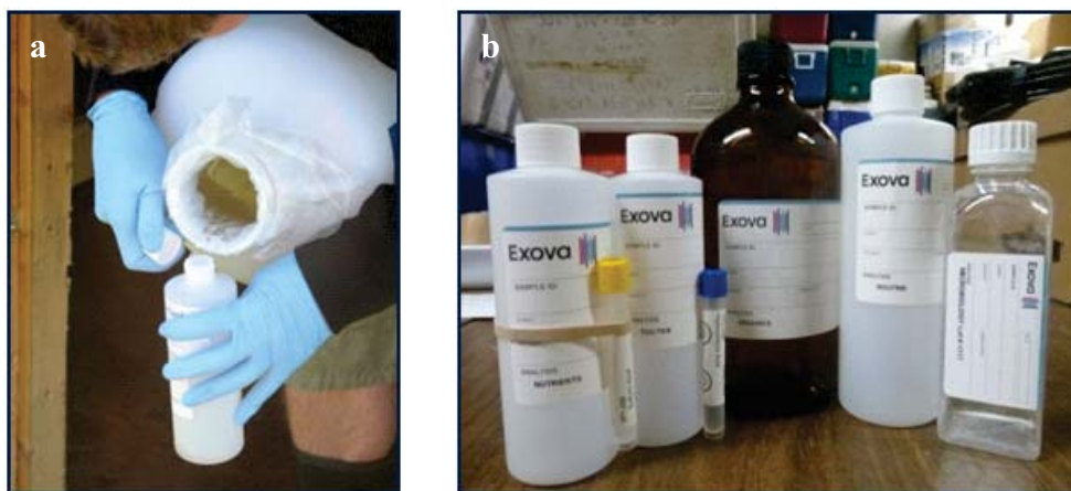
Figure 2.26. Water samples being (a) sub-sampled in the field and (b) bottles for specific lab analysis.
