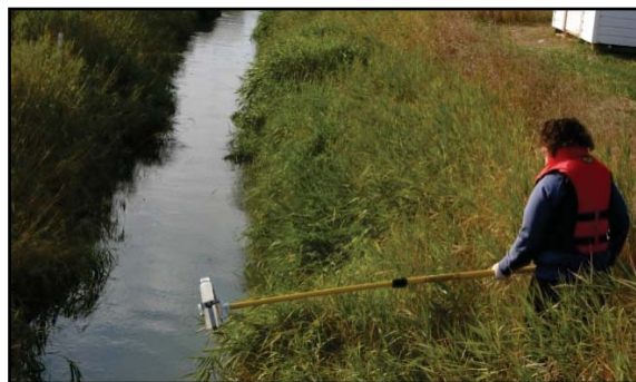
Figure 2.25. Grab sampling with a pole and sample bottle at the Battersea Drain Field.
