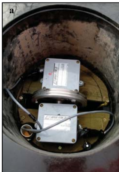
Figure 2.15. Water stage in the circular flumes was recorded using (a) two float potentiometers, with one connected to a (b) Lakewood datalogger used as a backup
