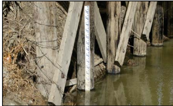
Figure 2.19. Staff gauge attached to the bridge at Station 23 in the Indianfarm Creek Watershed.
