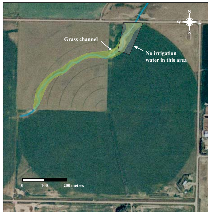
Figure 6.2. The grass channel and zone of no irrigation application beneficial management practices implemented in the east quarter section at the Lower Little Bow Field.
