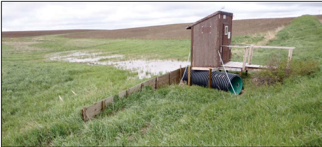
Figure 6.6. Rainfall runoff entering the flume at the edge-of-field monitoring station at the Lower Little Bow Field on May 28, 2010.
