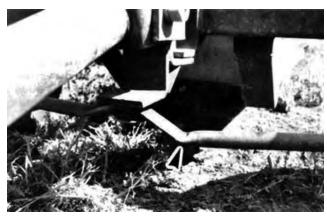
FIGURE 5. Bent Steering Tie Rod.
