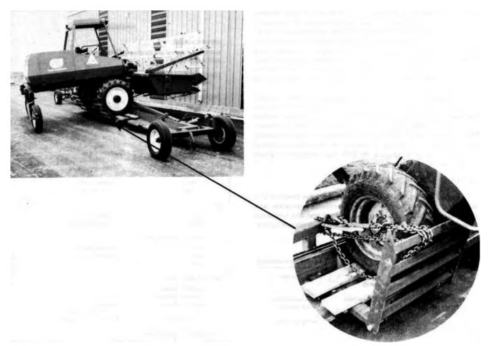
FIGURE 4. Loaded Windrower Illustrating Tie-Down Procedure.
