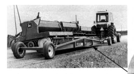
FIGURE 2. Doepker Transporter Loaded with Three Press Drills.
