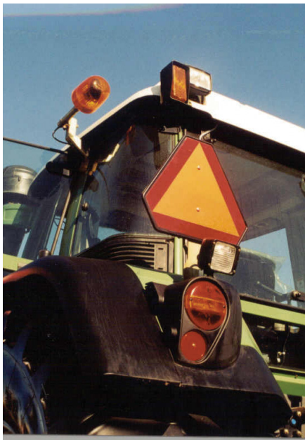
Machinery travelling slower than 40 km/h must have a slow moving vehicle sign attached to the back of the self-propelled farm equipment and any towed implement.
