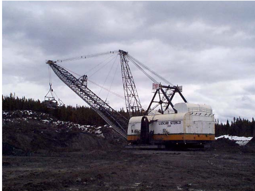
Figure 3 Dragline used to remove the overburden to expose the coal seam
