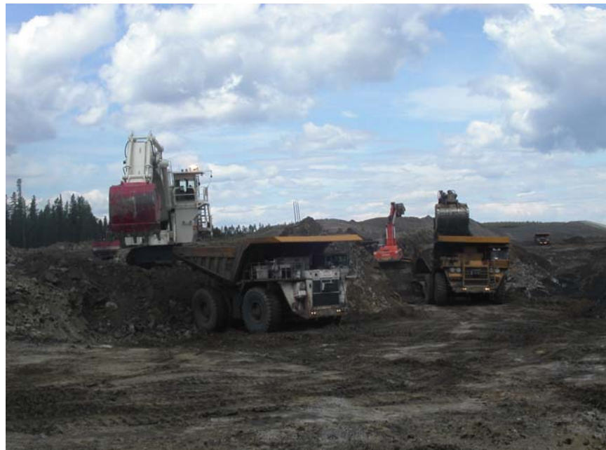
Figure 4 Large backhoes used to load haul trucks
