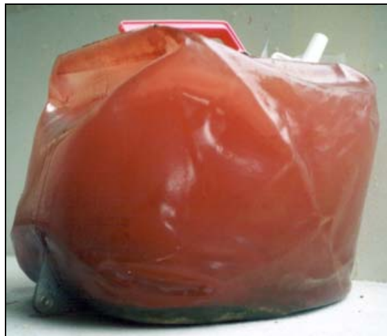
Figure 1. Elemental selenium formed by bacterial reduction of selenate.
