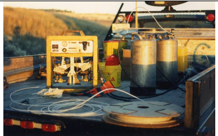
Epoxy resin pressure injection pump and component injection tanks.
