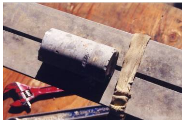
Concrete cores may be required to determine color changes and to perform petrographic analysis and compressive strengths.
