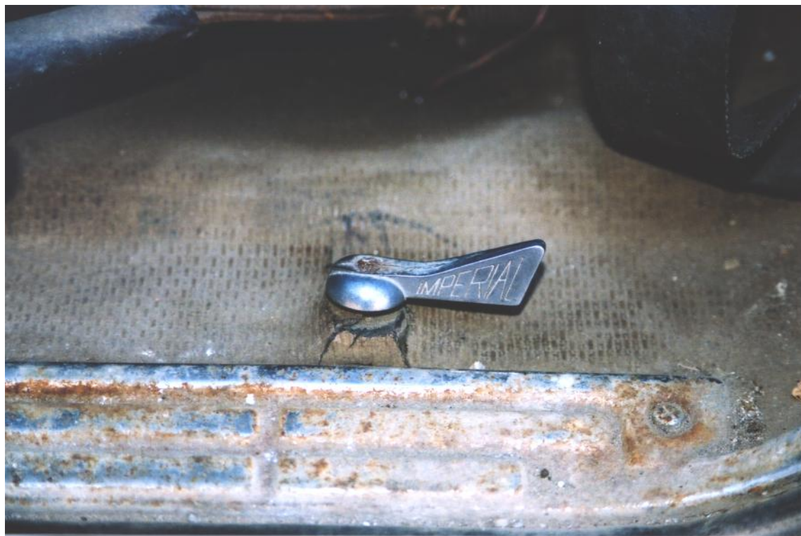
Photograph 9: Shows the 3 way valve turned to open gasoline flow from the passenger's side gasoline tank.
