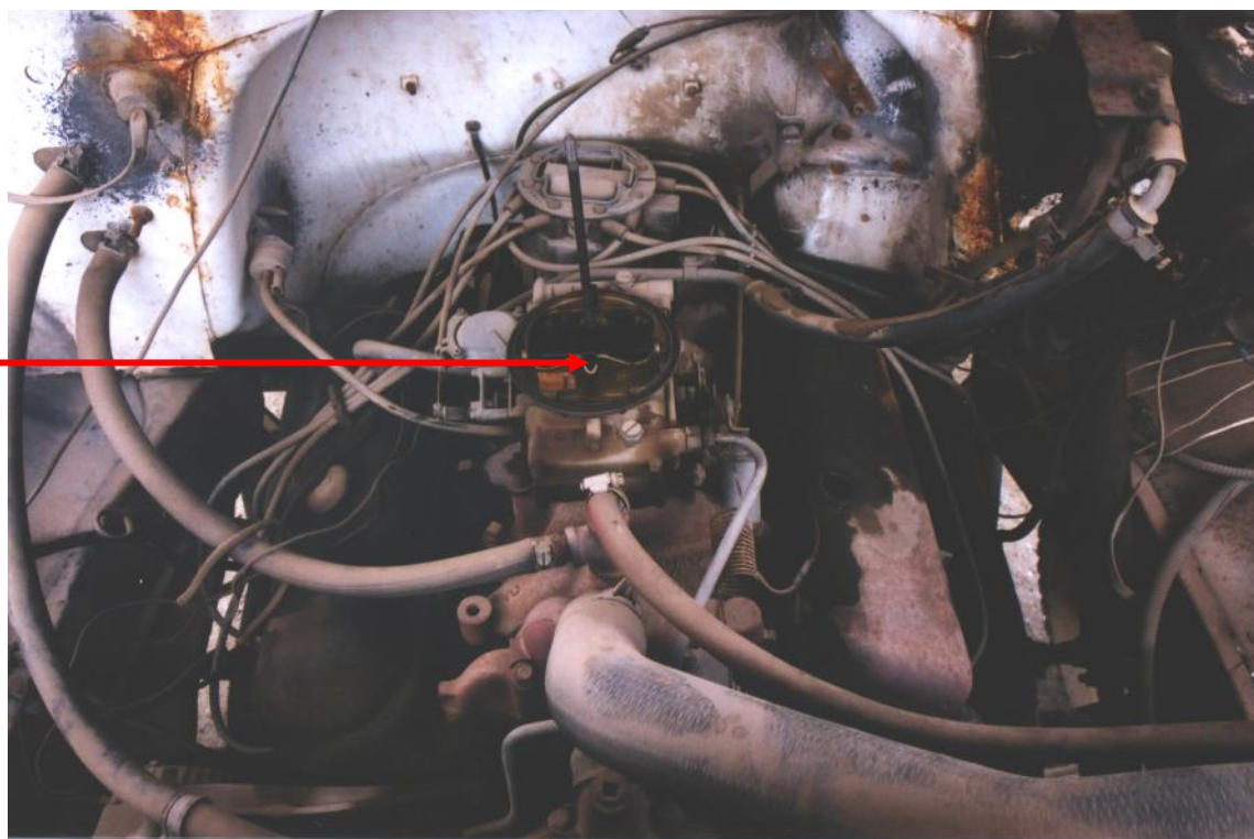
Photograph 6: Shows the twin barreled carburetor to which gasoline was poured.
