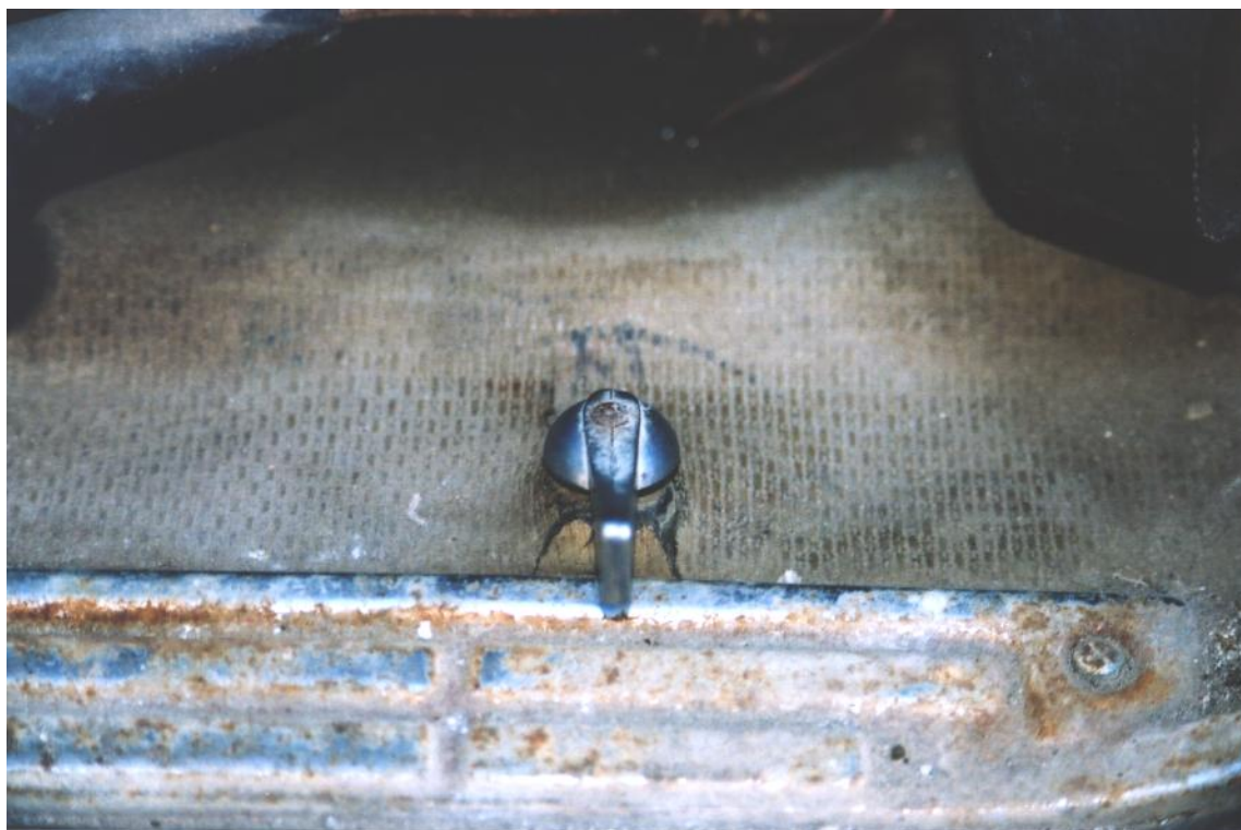
Photograph 8: Shows the 3 way valve turned to open gasoline flow from the driver's side gasoline tank.
